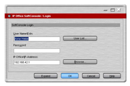
In the **USER NAME** field, enter your extension number or user name as it is programmed in the telephone system. The user name is case sensitive.
