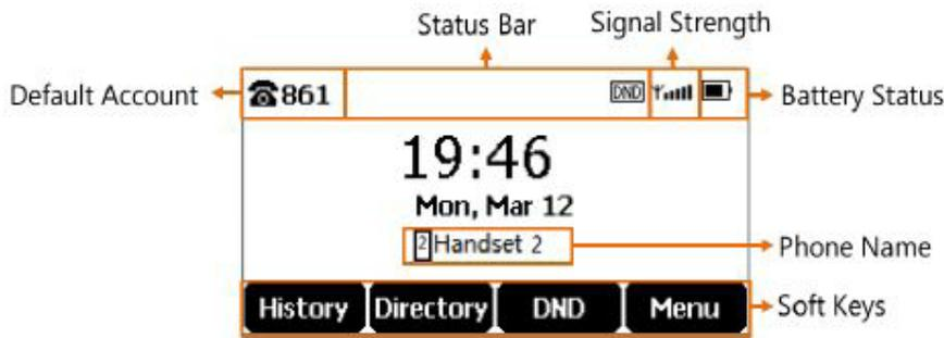
The idle screen is made up of the signal strength, battery status, status bar, phone name and Softkeys.
