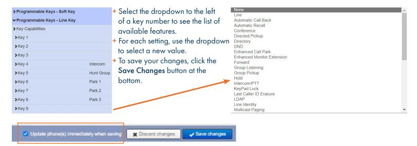
**NOTE**: When the box shown above is checked, the phone will reboot immediately upon save. Uncheck the box to have the phone reboot overnight.
