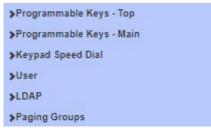
NOTE: For the Mitel 6867i, in the **Programmable Keys Top** section, you should only program keys 6-20 as the first 5 keys are standard features across all Business Groups. In the **Programmable Keys Main** (Softkeys) section, keys 6-18 are programmable as the first 5 keys are standard features across all Business Groups.
