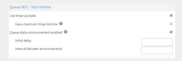
Set both the initial delay (the time before the first announcement is played) and the interval between announcements in **seconds** between 0 and 300.
